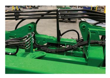
If the customer did take advantage of the factory option, we also have kits that can update the Deere OEM manual/setpoint system to our LDM ISOBus/setpoint system. Our update kit installs in just a couple hours, swapping the control valve cartridge to a PWM style and adding our ISOBus controller and wire harness tie-in. With this update kit, the customer can easily enjoy all the benefits of in cab ISOBus control with their existing system.
